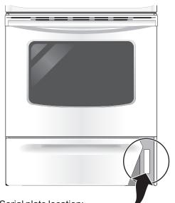
Serial plate location; Open storage drawer (some models) or remove outer lower panel (some models).
